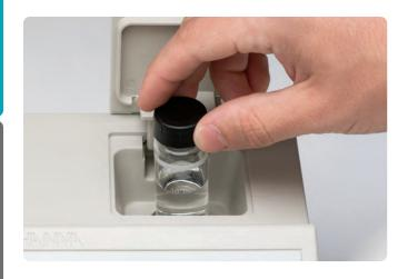
All measurements are performed with 25 mm round cuvettes composed of special optical glass to ensure maximum repeatability of turbidity and chlorine measurements.
